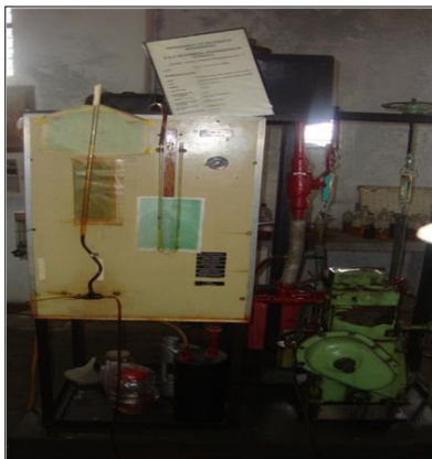
Fig 1: Single cylinder water cooled 4 stroke diesel engine
